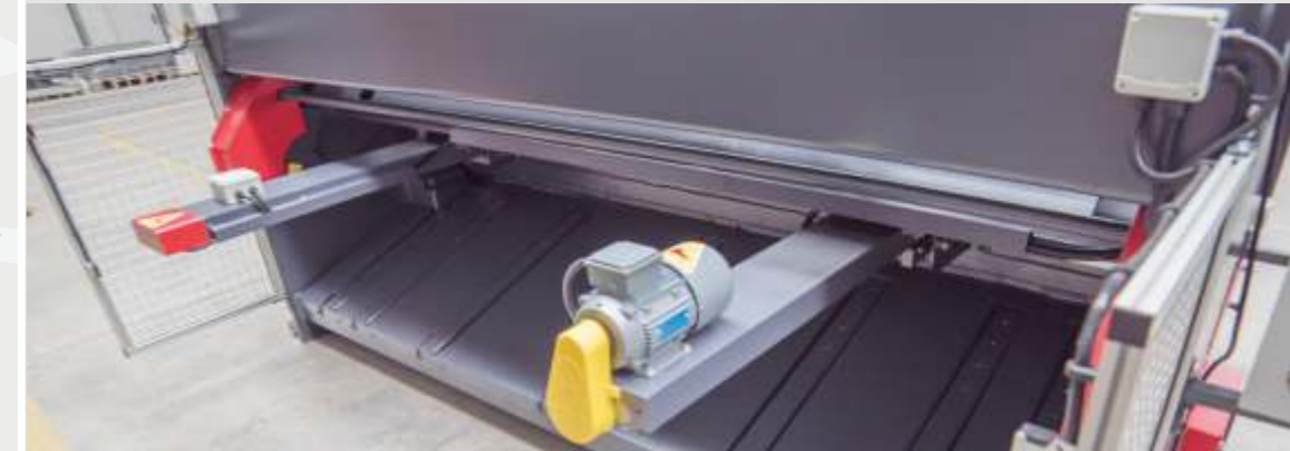
Motorized Back Gauge has \pm 0,1 mm Accuracy
