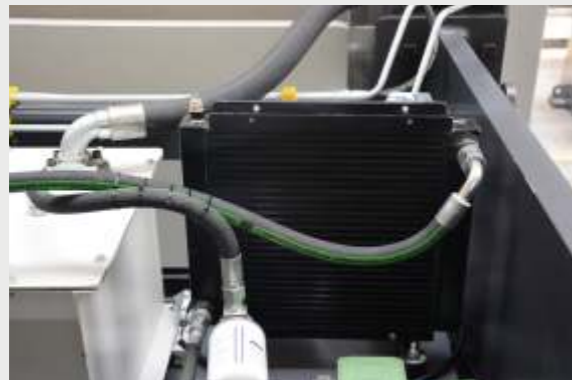
Hydraulic Oil Cooler System
