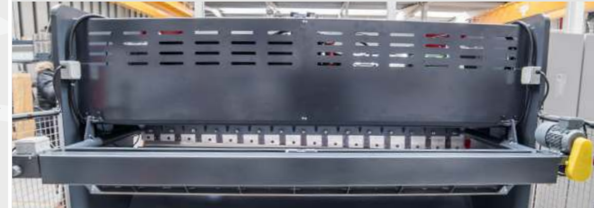
Motorized Back Gauge has \pm 0,1 mm Accuracy
