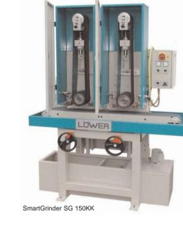
SmartGrinder models with one or two sations use the same machine frame. This way the second unit can be fitted to a single unit machine even at a later date.
